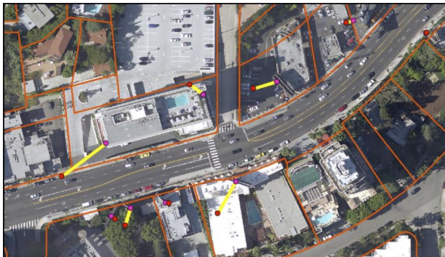
Figure 4. Sample image of ArcMap with line measurements between web and field data points.
