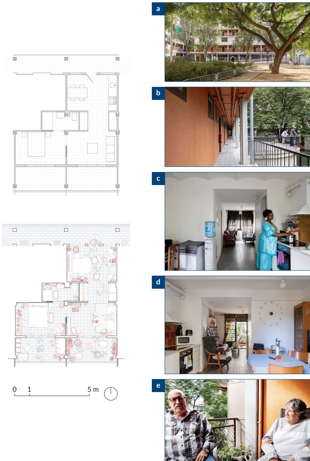
Figure 3. The Casa Bloc case study houses general applicants and social emergency groups. On the left, the floor plans as built (top, redrawn) and post-occupancy (below) are presented. On the right, the photographs are by Adrià Goula ([a], courtesy of Adrià Goula) and Maite Caramés ([b–e], in Figuerola & Bilbao, 2023, pp. 197 [e], 199 [c, d], 201 [b]), 2022.
