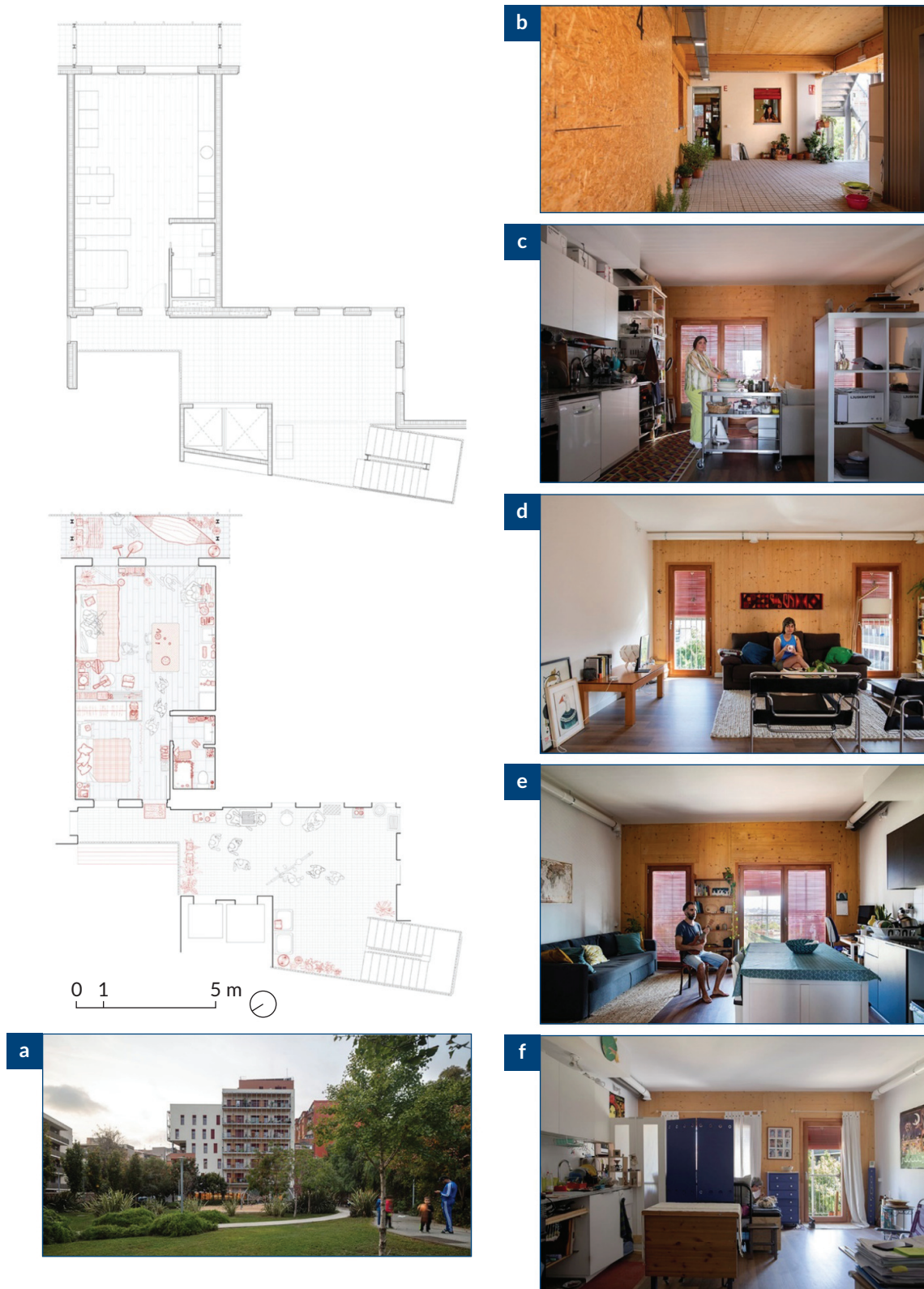
Figure 5. Cirerers cooperative housing case study. On the left, the floor plans of one shipping container unit as built (top, redrawn) and post-occupancy (below) are presented. On the right, the photographs are by Adrià Goula ([a], in Figuerola & Bilbao, 2023, p. 149) and Maite Caramés ([b–f], in Figuerola & Bilbao, 2023, pp. 152 [e], 153 [d], 154 [c, f], 157 [b]), 2022.
