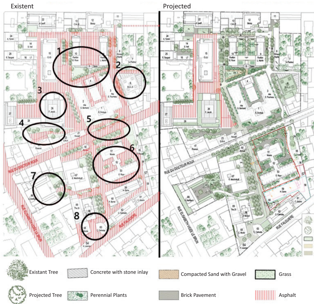
Figure 2. Comparison between the existing state of the chosen site and the intervention plan. Source: Courtesy of AIA Life Designers.
