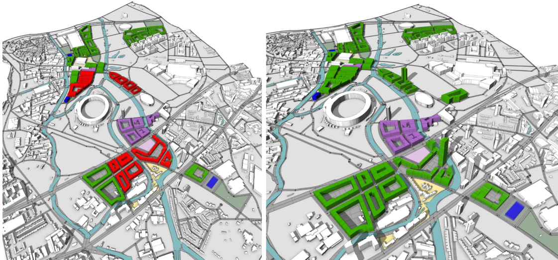
Figure 4. Let's assume that the employment of a nearby university zone is tripled. The demand in the residential area calculated by QUANT shows that it exceeds the building's capacity and is indicated using red volumes (weighted distribution considers proximity to the university). On the left side, we created two skyscrapers based on permitted development zones in the planning applications. New scenario capabilities allow the user to experiment with multiple solutions/variations that satisfy the population projections, e.g., experiment with building density scenarios.
