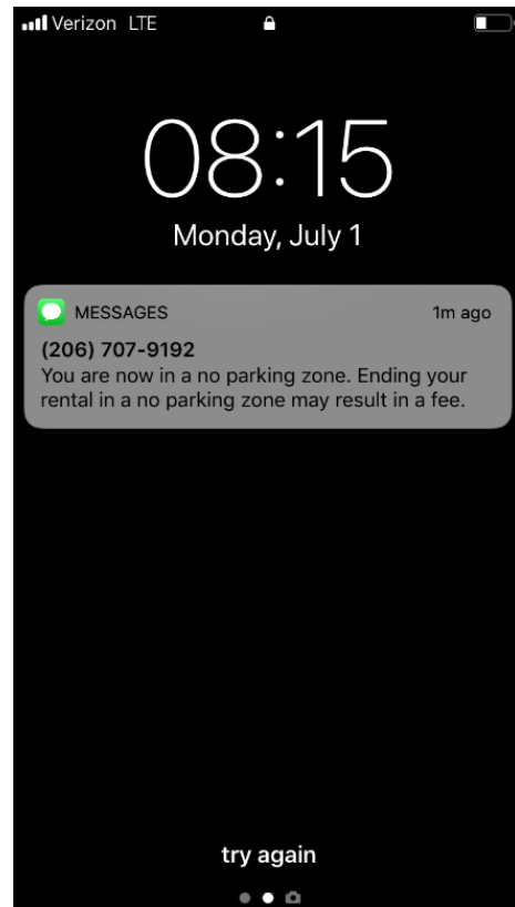
Figure 4. An SMS notification to a bike share rider upon entering a geofenced no-parking zone. Source: Author.
