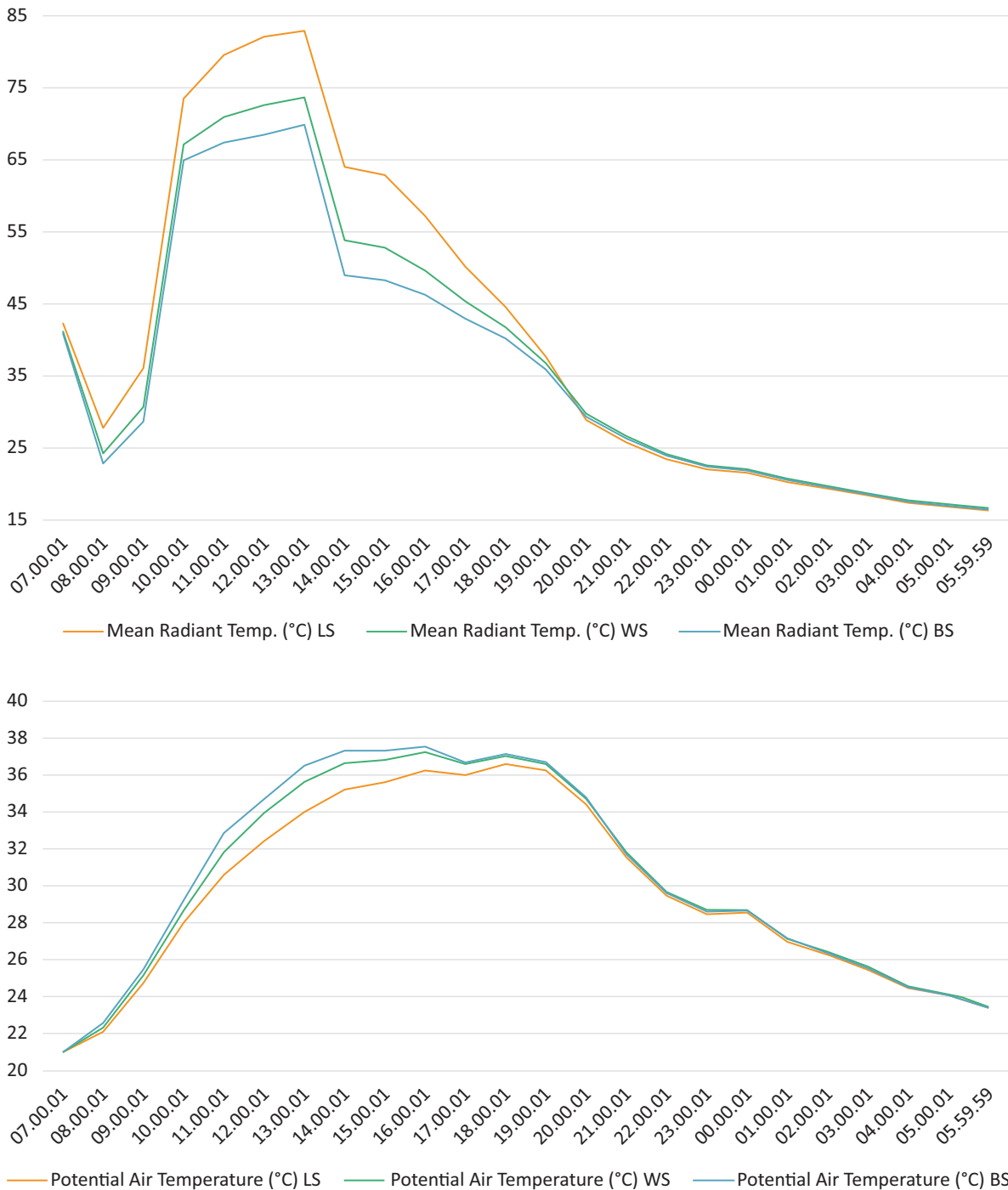
Figure 7. Comparison of the influence of surface albedo on the PAT for an entire day of simulation using ENVI-met software. Notes: LS = light surface (albedo = 0.8), BS = black surface (albedo = 0.2), WS = wet surface (albedo = 0.4).
