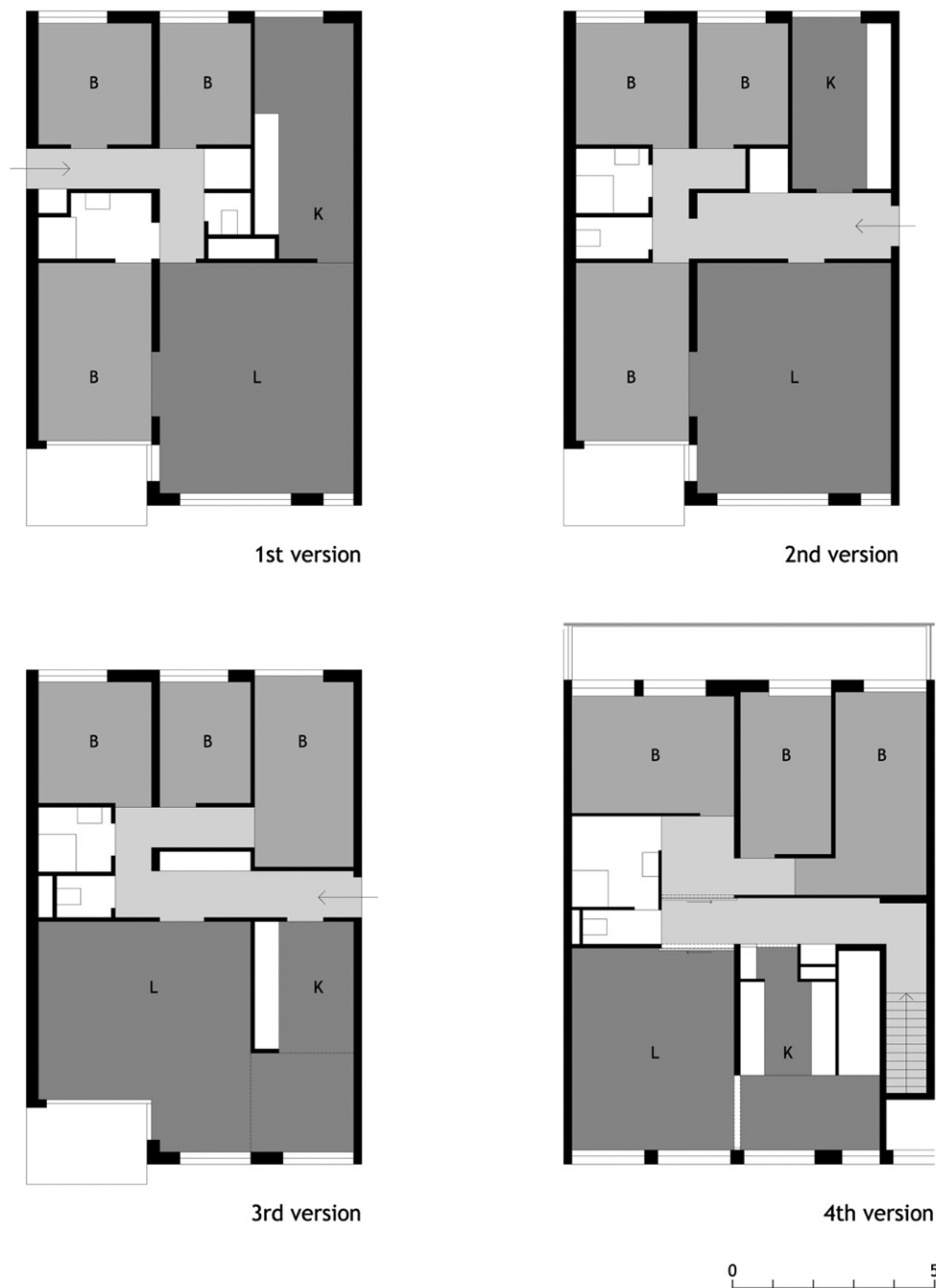
Figure 8. Evolution of the layout of the floorplan for the apartments in the Punt en Komma blocks. Author’s drawings.
