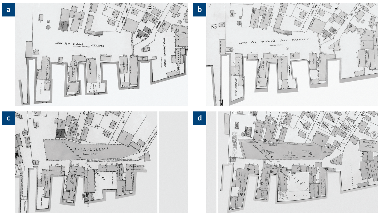
Figure 8. Evolution of the John Pew & Son processing plant. Notes: (a) 1892; (b) 1898; (c) 1903; (d) 1919; this figure is adapted from data in the Collection Sanborn Maps (Sanborn Map Company, 1888–1949).
