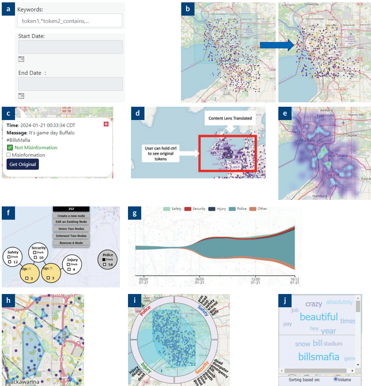
Figure 4. Visualization features: (a) keywords and date filters; (b) spatial filter; (c) tooltip; (d) content lens; (e) heat map; (f) classifier nodes window; (g) theme river chart; (h) cluster view; (i) cluster lens; (j) topic cloud.
